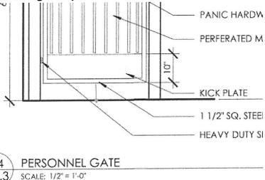
3<sup>rd</sup> review comment: Sheet A1.1, dimension strike edge clearance on the pull side of gate. Shall be minimum 24 inches at exterior gate. [Response indicates 18 inches of strike edge clearance only]
